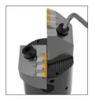
**Step 1:** Loosen the mounting screws on both cartridges.
