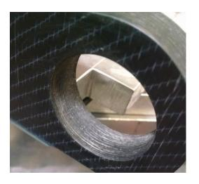
Allied Machine Solution: Carbide Clad Special Helical Holder with Diamond coated T-A® drill insert
