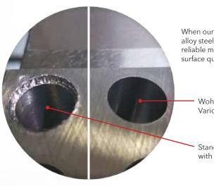
When our customer was machining alloy steel to 9xD, the  $NOVI^{TECH}$  provided reliable machining, which achieved high surface quality (Ra = 1  $\mu$ m).
