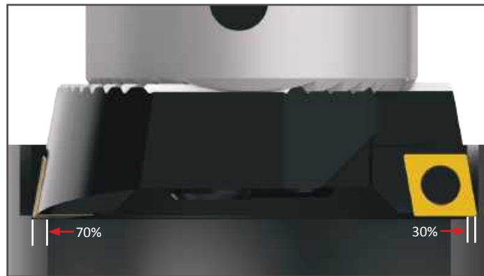
Material removal up to 7.00 mm - 10.00 mm on diameter: 70% roughing 30% finishing
