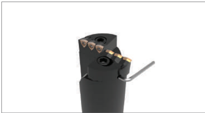
Step 3: Set the diameter using the adjustment screw against the mounting screw. Place the drill in a pre-setter to ensure the correct diameter setting.
