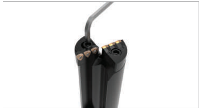
Step 4: Tighten the mounting screw to 11-14 ft-lbf (15-19 N-m).
