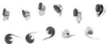
Periphery edge chip formation:
