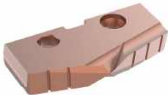
150° Structural Steel For material over 7/16" thick and for reduced exit burr.
