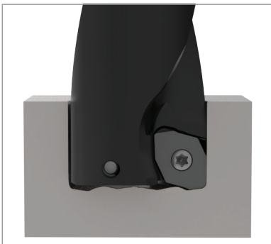
Periphery edge chip formation:
